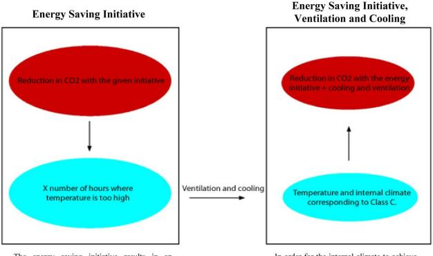
The energy saving initiative results in an increase in the number of hours where the temperature is above a certain level. This results in an internal climate which is worse than that recommended by the Working Environment Authority, Class C.
