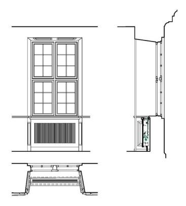
The traditional heat risers were replaced with a hidden supply in the floor. This was only possible as the floor was already being replaced.
