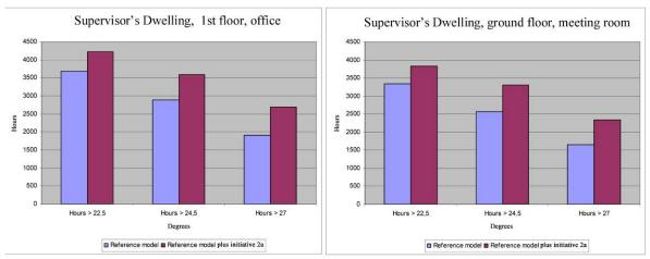
The graphs above show the number of hours where the temperature is over a specified temperature in, respectively, the first floor office and the ground floor meeting room.
